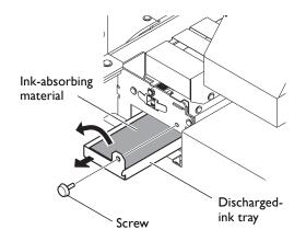
Secure the discharged-ink tray in place and re-attach the side cover.
